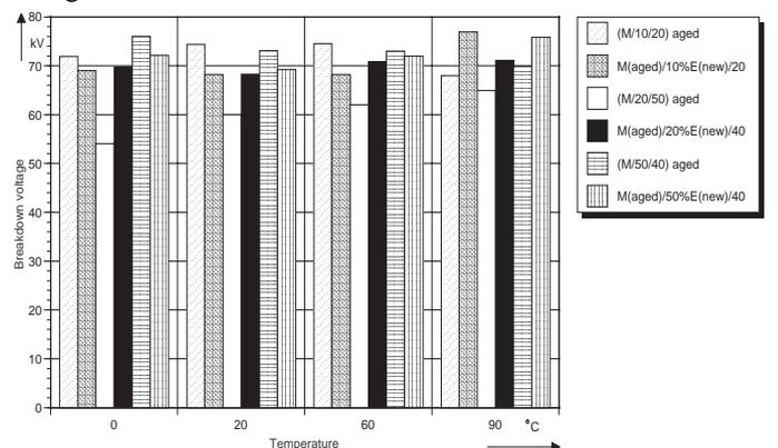
Figure 6 - Electrical strength of aged and new ester liquids / mineral oil mixtures
