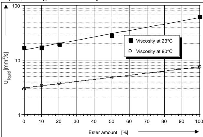
Figure 7 - Viscosity of ester liquid/mineral oil mixtures at different temperatures
