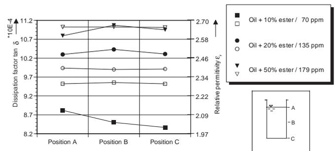
Figure 1 - Dissipation factor of different mixtures of mineral oil and ester liquids
