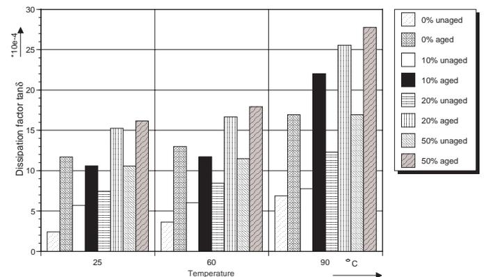
**Figure 2** - Dissipation factor of new and aged ester liquid/mineral oil -mixtures
