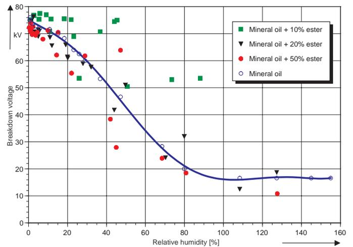
Figure 5 - Comparison of the breakdown voltage of the liquid mixtures with that of mineral oil
