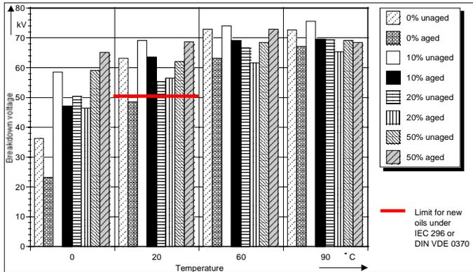
Figure 3 - Breakdown voltages of new and aged mixtures of ester liquid and mineral oil
